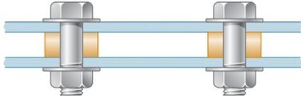
Two steel plates are to be held together by means of 16-mm-diameter high-strength steel bolts fitting snugly inside cylindrical brass spacers. Knowing that the average normal stress must not exceed 200 MPa in the bolts and 130 MPa in the spacers, determine the outer diameter of the spacers that yields the most economical and safe design.
